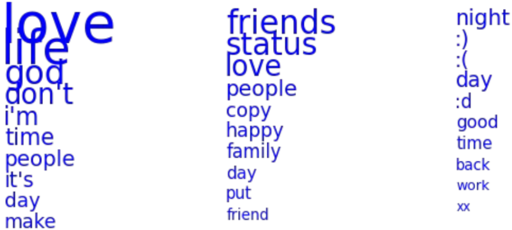
Figure 3.1: Sample set of LDA topics inferred from user status updates on Facebook using LDA with 10 topics (LDA10).
